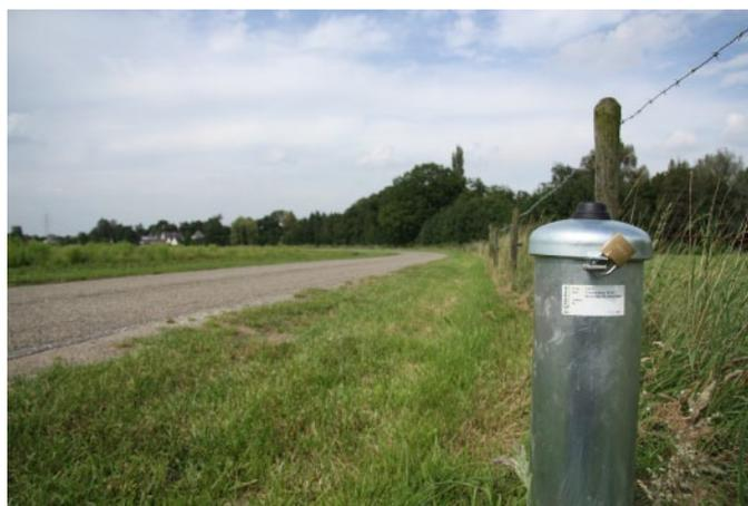
What equipment was delivered by Eijkelkamp 47 measurement locations were set up and equipped with Diver water level loggers and e-SENSE monitoring well modems for Doetinchem council. This modem, in combination with a pressure transducer in the monitoring well, records the correct rise height in relation to mean sea level. Every day the data is automatically sent to the council's central main station. The same data
